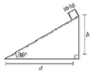
2. What is the normal force and the parallel force of 10 kg block sitting on a  $40^{\circ}$  incline?
