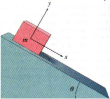
3. What is the normal force and the parallel force of 10 kg block sitting on a 10° incline?
