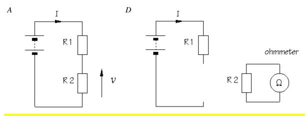
to measure resistance, the component must be removed from the circuit altogether
