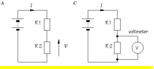
to measure potential difference (voltage), the circuit is not changed: the voltmeter is connected in parallel
