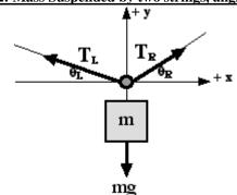
**<u>Calculation 2</u>**: Using the expression you derived in Calculation 1, complete Table 1. System 2: Mass Suspended by two strings, angles unequal.
