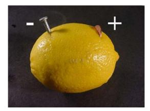
This is a single cell of a battery. The zinc nail and the copper penny are called <u>electrodes</u>. The lemon juice is called <u>electrolyte.</u>
