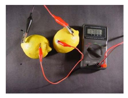
The two lemon batteries above, combine to produce a voltage of 1.788 volts. This combination still does not create enough current to light a small bulb. Note the red wire connecting the batteries is joined from "+" (penny) to "-" (galvanized nail).
