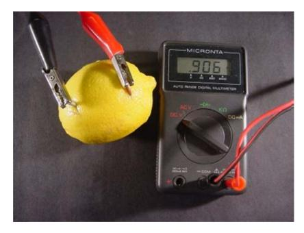
To solve this problem we can combine battery cells to create higher voltages. Building more lemon batteries and connecting them with a metal wire from "+" to "-" adds the voltage from each cell.
