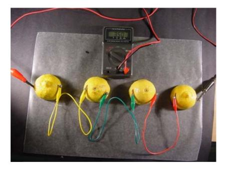
Four lemon batteries create a voltage of 3.50 volts. We should be able to light up a small device like an LED (Light Emitting Diode).
