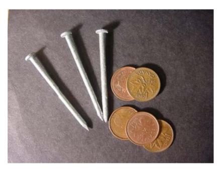
**Creating the battery**: Insert a penny into a cut on one side of the lemon. Push a galvanized nail into the other side of the lemon.
