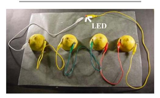
In the above image, electrons flow from the "-" (nail) end of our lemon battery through the LED (making it glow) then back to the "+" (penny) end of the battery. This is an electronic circuit. The LED glows **dimly** with this configuration.
