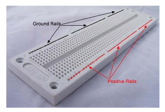
To build a circuit, simply push components or wires into the tiepoints. Components such as integrated circuits in a DIP packages can be placed in the middle of the boards with legs on either side of the conter groove. The photo below shows a simple LED circuit.
