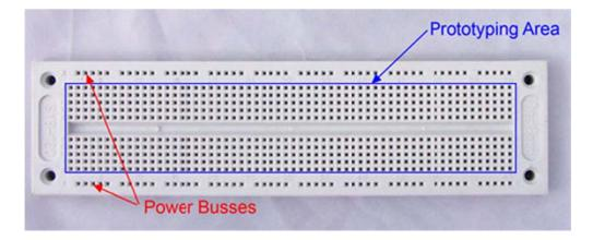
The tiepoints in the prototyping area are typically arranged in groups of 5 which are connected together. These are referred to as terminal strips and are shown in the photo below...
